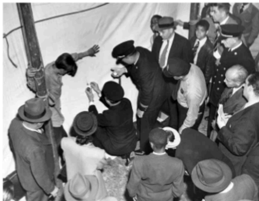
Prior to the Ringling Brothers and Barnum & Bailey performing under a new, fireproofed canvas for the 1945 season, Washington, D.C. fire marshal R.C. Roberts holds a match to the sidewall as deputy fire marshal Captain R.A. Warfield holds a stop watch, measuring the time that the canvas remains burning when the contact with the flame is removed. Photo by Acme Photo, from author's collection.
